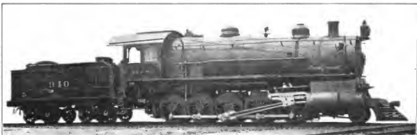
Fig. 47. Decapod (2-10-0) Tandem Compound Locomotive. Built by the Baldwin Locomotive Works for the Atchison, Topeka & Santa Fe. Cylinders 19 in. and 32 in. x 32 in., Working Steam Pressure 225 lbs. per sq. in., Total Heating Surface 5,200 sq. ft., Diameter of Drivers 57 in., Weight on Drivers 237,800 lbs., Total Weight 267,800 lbs.
